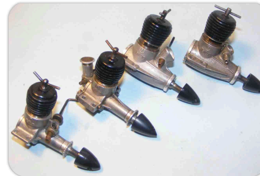
7. Below The German Taifun 1cc Hobby was the baby of the Taifun range. All four versions are shown here.
