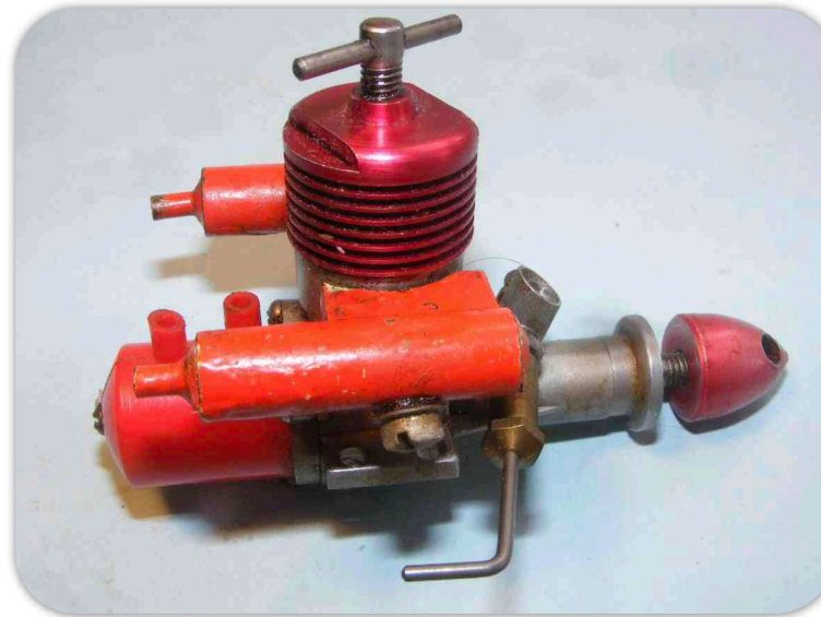
4 Above. The 1cc ME Heron, introduced in 1960 by IoM-based Marown Engineering. This is a later model with nylon tank, earlier ones had a red anodised red tank.
