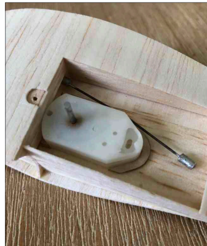
Mike Mulholland's Twin Fin with detail of folding propeller and Tomy DT timer. Full coverage of Mike's immaculate build is in the AMAC Slipstream, April 2023.
