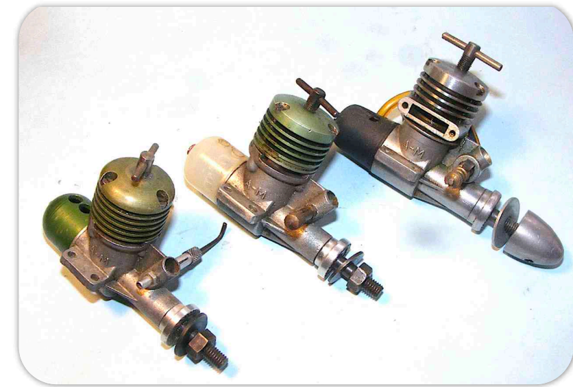
5 Above. 1cc AM diesels. Mk 1, Mk 2, and the final Premier Plastics version. The last was also available as a glow plug engine.
