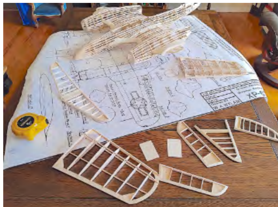
OPPOSITE: Views to show the way in which central wing spars merge into nacelle and fuselage formers to make a tight unit.
