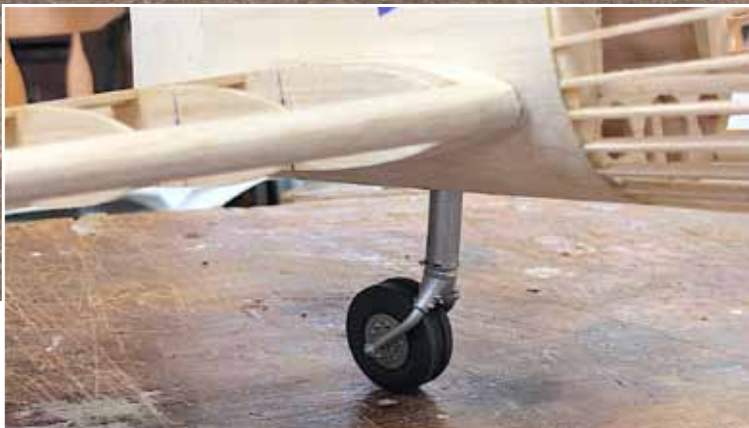
LEFT: The tailwheel assembly detail.
