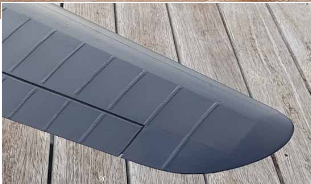
ABOVE: Wing details showing lightweight covering, and tape and stitching simulation.
