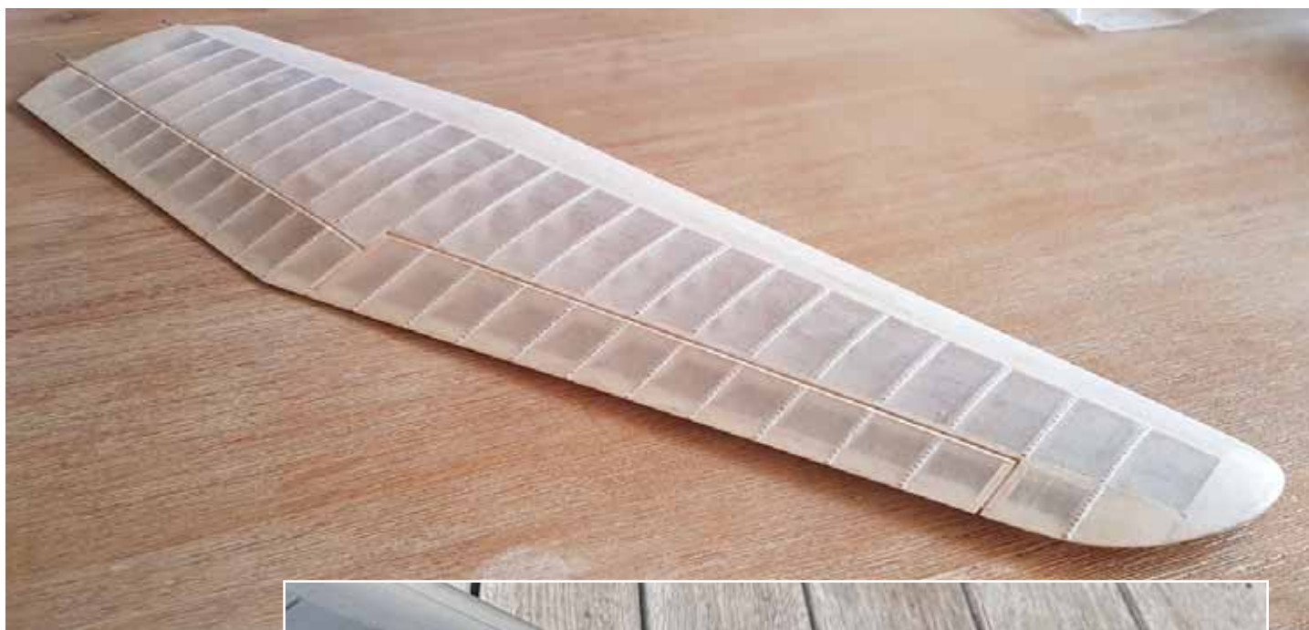
ABOVE: Wing details showing lightweight covering, and tape and stitching simulation.
