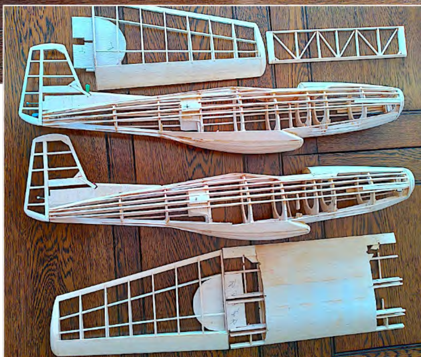
TOP AND RIGHT: Views of the model showing the construction of the plug in-knock-off wings and sheeted centre-section and unusually, two fuselages to build!
