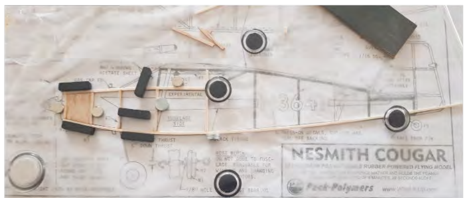
ABOVE AND RIGHT: Building progress showing magnets in lieu of pins, and notice board used as a building board.
