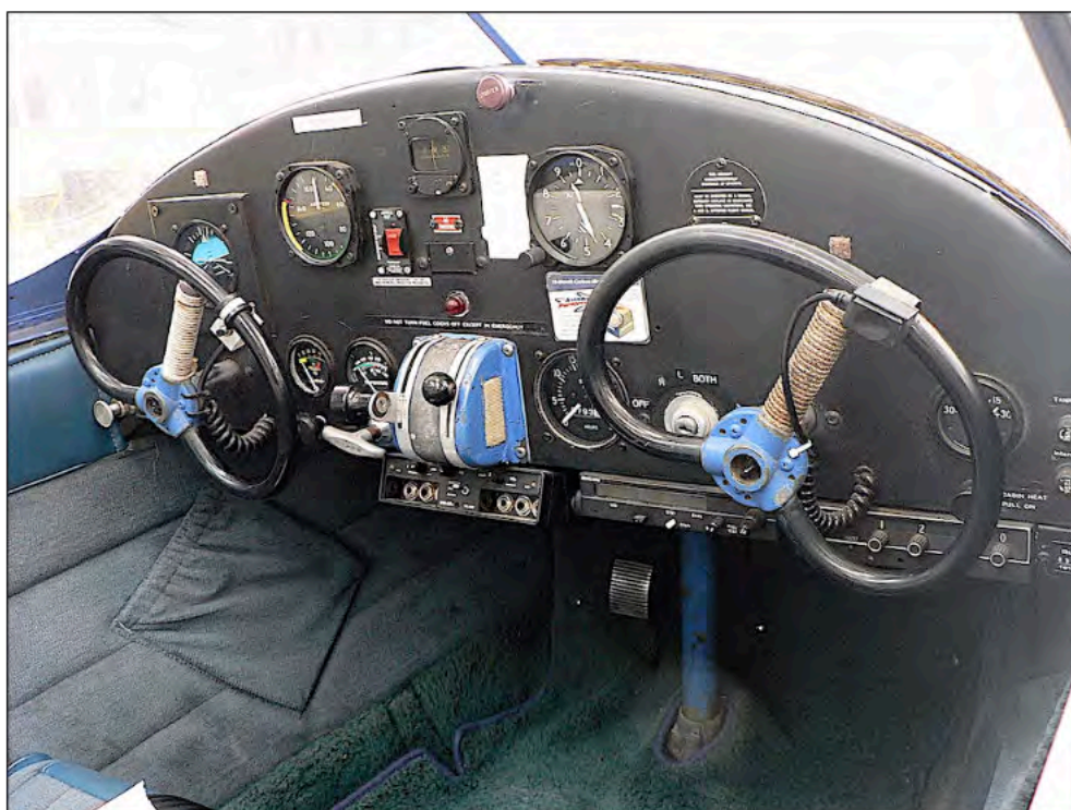
RIGHT: A cockpit view of the Ercoupe reveals an absence of rudder pedals.
