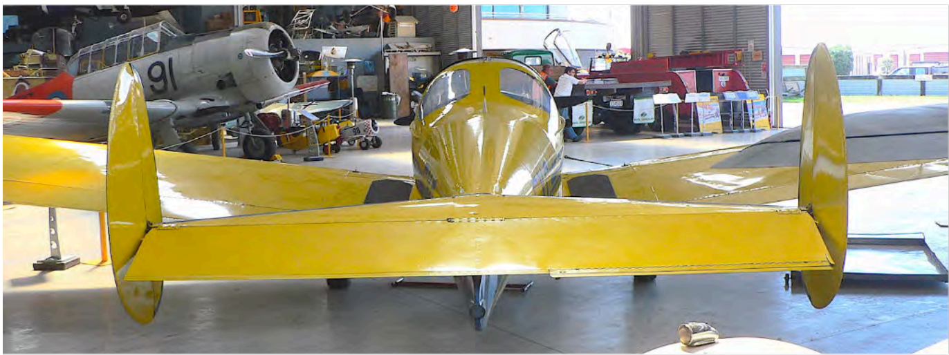
ABOVE: Several views of the Ercoupe that show the marked dihedral it has.
