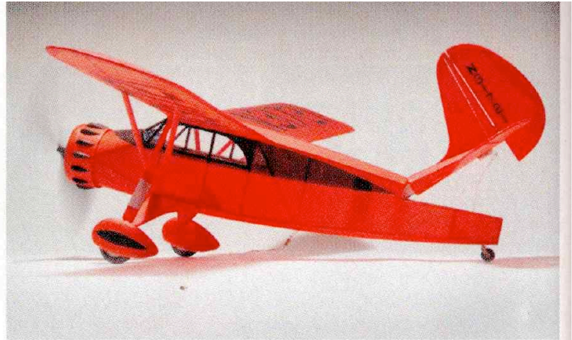
entire rudder and stabilizer unit to a 45-degree angle. It is actuated by a hidden viscous timer on the underside of the beautifully rendered craft and a small music wire spring embedded in the structure at the leading edge of the stabilizer.
