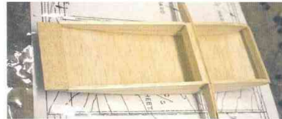
The ply dihedral brace is fitted ready for building the outer panels...
