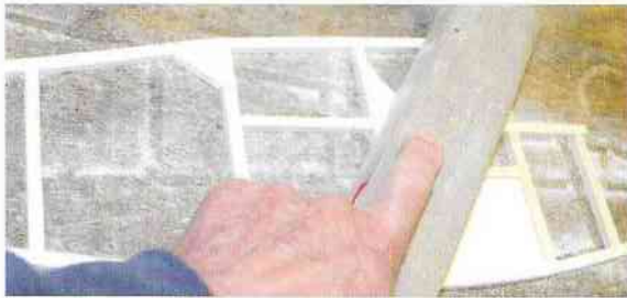
Sand the 'rough' side of the fuselage sides before joining.
