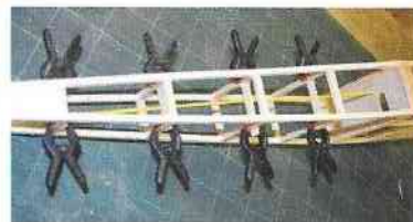
Fixing supports for the elevator control shake
