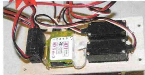
Radio installation plate is screwed to bearers on the fuselage. The rx is fitted on the bottom of the tray.
