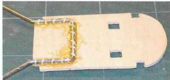
Bind and epoxy the pianowire undercarriage to former F1.
