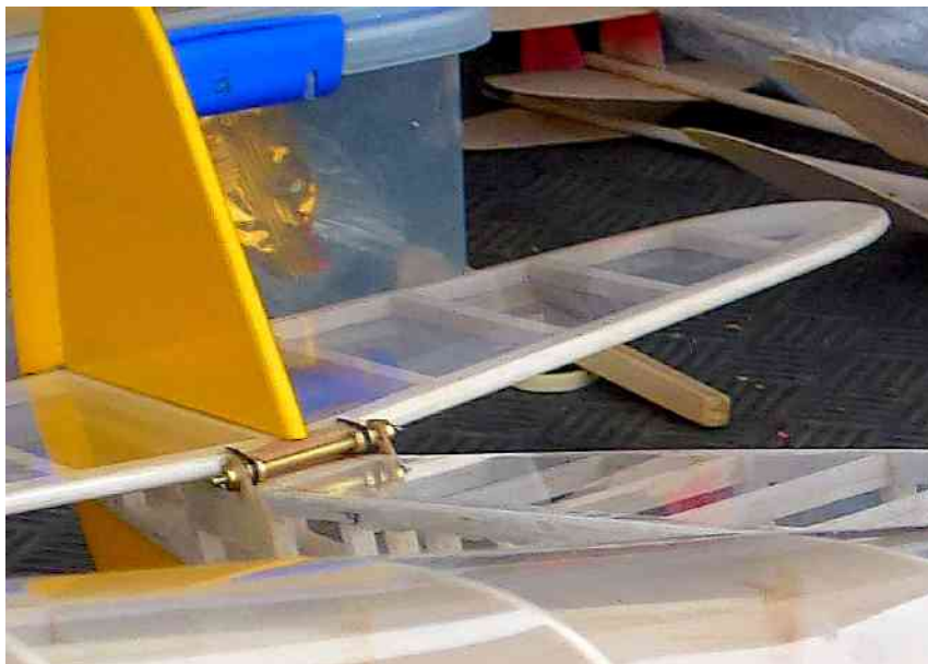
Below: Stylish tailplane hinges engineered by Julius Long for his Simplex models.
