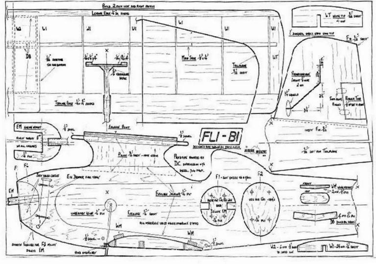
The *FLI-BI* An Australian design that takes the Ebeneezer concept closer to efficiency with built-up wings.
