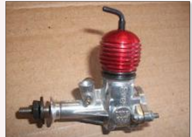
McCoy also experimented (as did OK) with diesel versions of their 1/2A motors. They used O-ring sealed contra-pistons which lacked the "feel" of conventional lapped diesels but which worked well enough in practice
