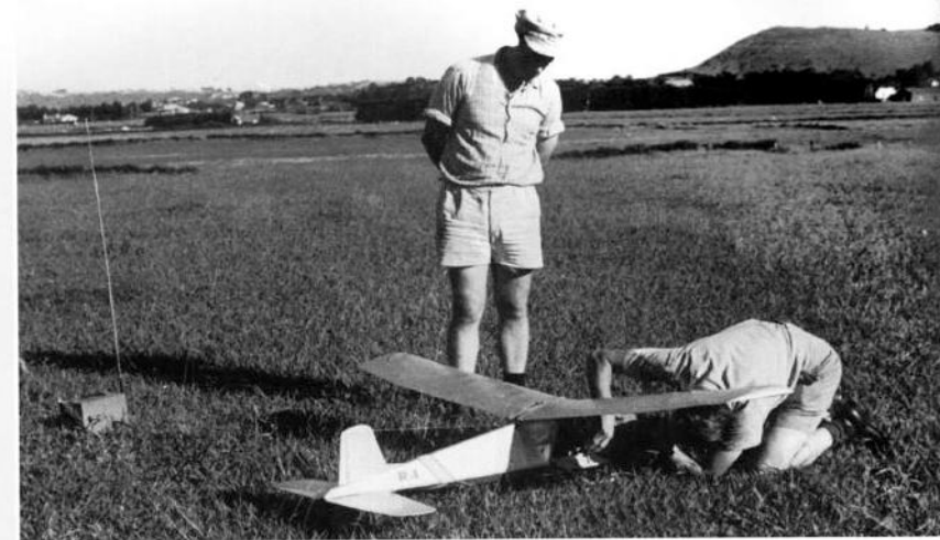
Below left: Frank Bethwaite winds the rubber motor of his Free Flight Wakefield model. Hamilton 1949/1950. Michael Taylor Photo
