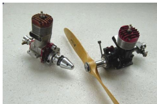
Photos above show the Carburettor modifications made by Bryan. It is good to read that the modification was successful and has resulted in a spark ignition motor that can be throttled in what is now a normal RC manner. The photo at the bottom right is two of Bryan's Spark ignition motors the one on the right being the Throttle fitted McCoy. (Photo by Neil McDougall all others supplied by Bryan Treloar)
